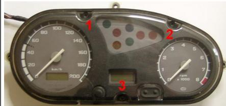
4/ Remove the three screws holding the front perspex cover
