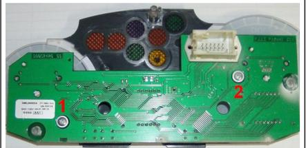
9/ Loosen the two screws holding the circuit board to the dash fascia
